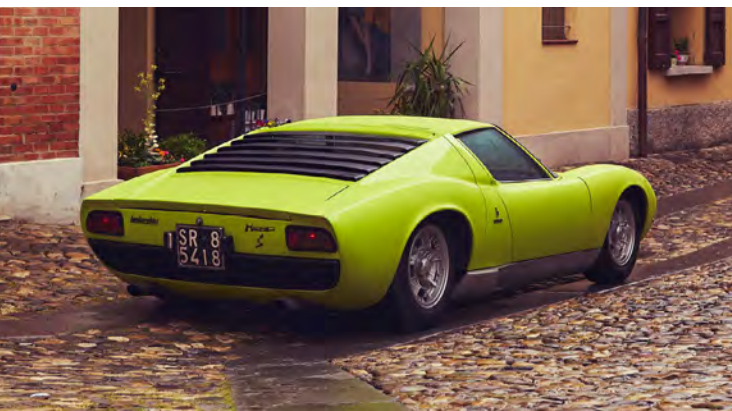
Considered the first real supercar, the Miura's raucous V-12 is located amidships, just behind the driver.
