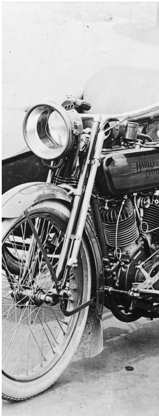
Prest-O-Lite attachment on a Harley-Davidson Model 18-F three-speed twin, circa 1918.
